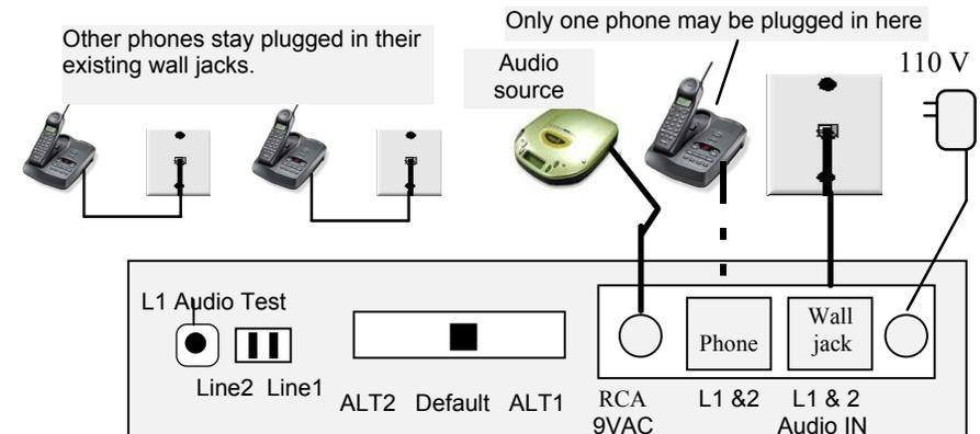
**Audio Test:** select L1 on your phone and press the **Audio Test** switch located in front of the SX2100EZ., you should be able to hear the audio. Adjust the volume to proper level or check the audio cord if needed to hear the audio. (Note: you can not perform audio test on line 2)
